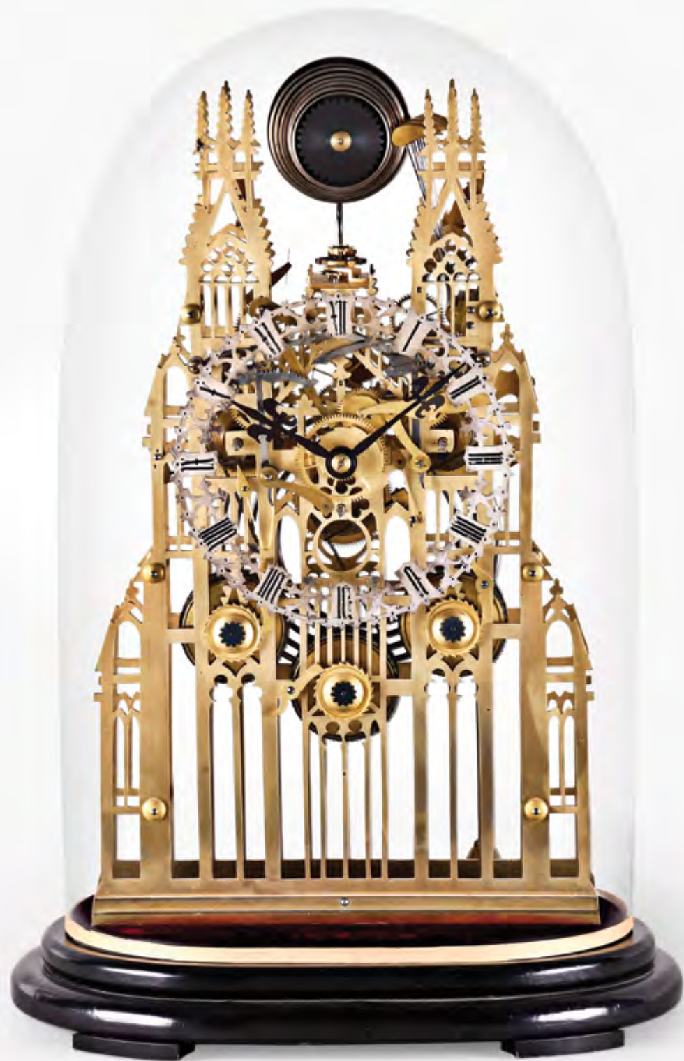
475 Attributed to Evans, Handsworth, a large York Minster skeleton clock, nicely fretted and finished brass architectural frames, fretted roman numeral silvered dial with blued steel fleur de lis hands, three train fusee movement with English lever platform escapement, uncut bimetallic balance, and six spoke crossings, chiming the quarters on eight bells aligned front to back between the towers, and striking the hours on a large gong, all mounted to a footed, velvet lined ebonized oval base, with conforming glass dome
