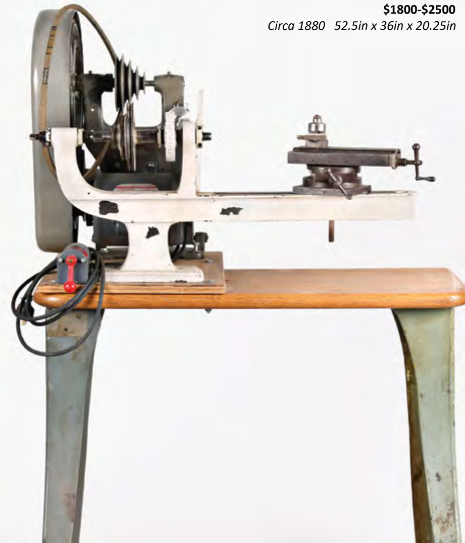
373 A late 19th century case maker's lathe, of white painted cast iron with 9 inch swing, 18 inch bed, and integral, plain bearing headstock with threaded spindle, screw feed tailstock with internal thread, chuck and center for tailstock, T rest, and screw feed slide rest, the lathe powered by a 1/3 horsepower motor, all mounted to an oak top bench with cast iron legs, and including many collets, ranging in size from 1 inch to 2 3/4 inches, with internal thread for attaching to the spindle, and external thread for the closer
