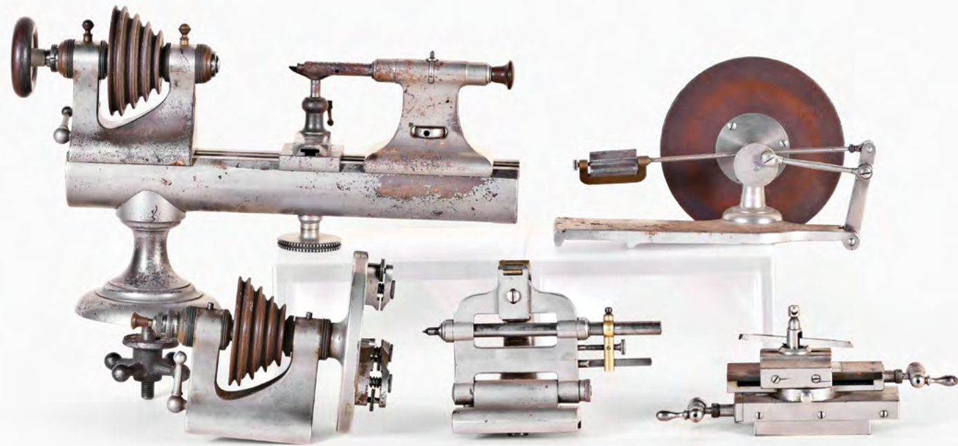
364 Ballou & Whitcomb, Boston, a very rare late 19th century watchmakers lathe with accessories, the lathe with 11 3/4 inch bed, 2 3/8 in. center height, T rest, plain bearing headstock accepting 8mm collets, an additional plain bearing headstock with integral faceplate, plain tailstock, jewelers tailstock, slide rest, and wig wag polisher
