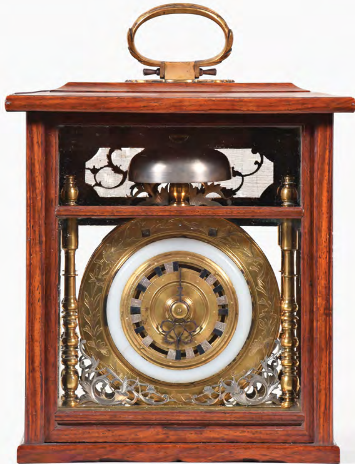
362 Japan, an early 19th century Makura Dokei with calendar, the polished brass frame with ornamental, turned pillars and silvered, engraved frets at the corners, the 30 hour, two train movement with round plates, turned baluster pillars and chrysanthemum engraving, verge escapement with six arm balance, count wheel striking on a bell, and calendar apertures above the rotating, white jade trimmed dial with fixed, blued steel hand and movable hour and half hour markers, in a shitan wood case having glazed, sliding front and back frames, silk backed sound apertures with pierced, engraved frets, and molded top with ornamental brass handle
