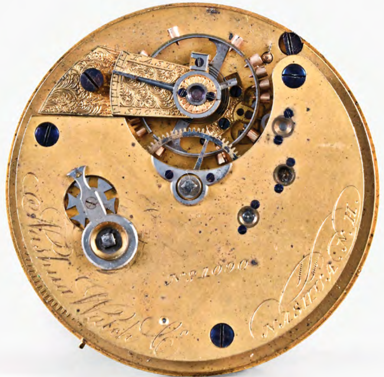
467 Nashua Watch Co., Nashua, N.H., a mid 19th century 20 size pocket watch movement, 19 jewel gilt plate movement with Stratton's safety barrel and maintaining power, Geneva stop work, and cut bimetallic balance with gold screws, and roman numeral, single sunk white enamel dial, serial #1090
