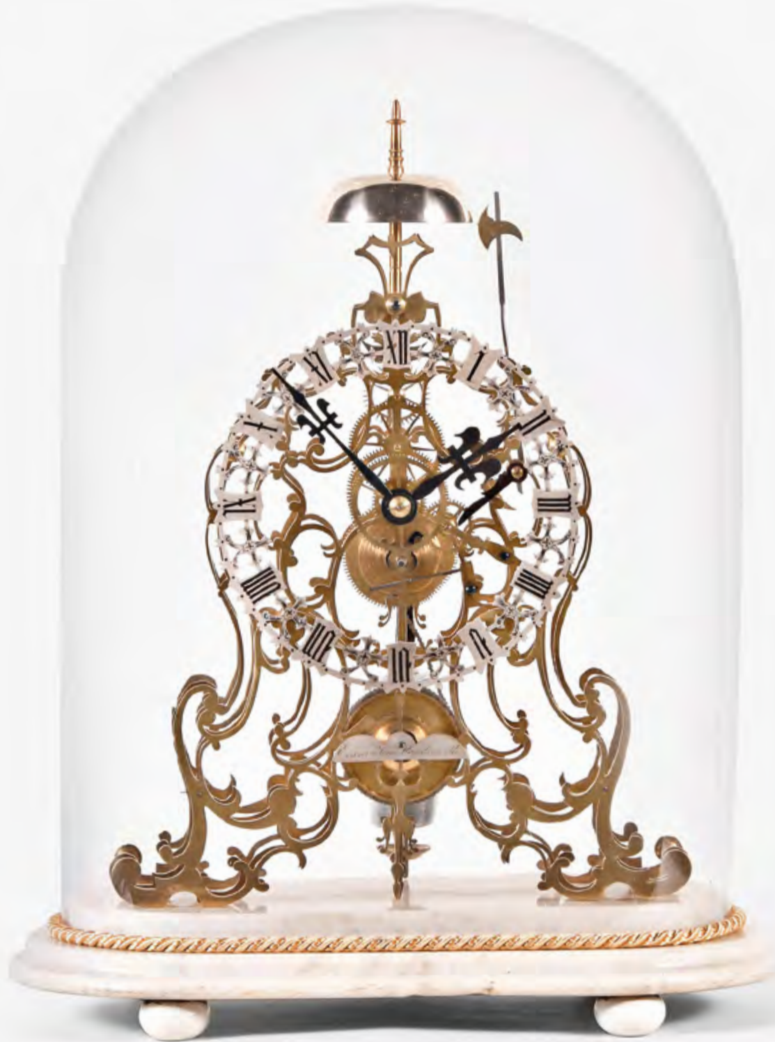
402 Evans & Sons, Handsworth, a fine mid 19th century arabesque skeleton timepiece, the well executed frames with seven pillars and fusee movement with wheels having six spoke crossings, recoil escapement, passing strike, and Evans compensated half seconds pendulum with cylindrical pewter bob, the skeletonized roman numeral silvered dial supported by a third fretted frame matching those behind, and with silvered plate engraved "Evans & Sons Handsworth", all resting on an oval, footed white marble base with conforming glass dome
