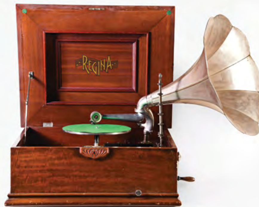
345 The Regina Co., Rahway, N.J., a scarce "Reginaphone" 20 3/4 inch disc music box with phonograph, mahogany case with molded base, short bedplate movement and duplex comb, removable cast iron platen and tonearm with horn for conversion to phonograph, serial #1260117
