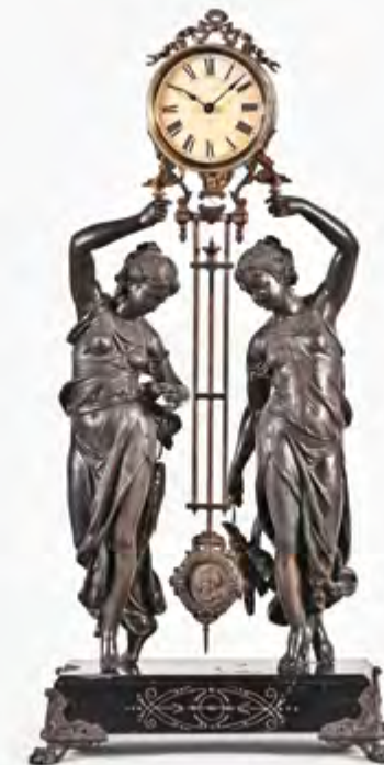
439 Ansonia Clock Co., New York, NY, "Crystal Regulator No. 4" mantel clock, gilt brass case with Royal Bonn top and base, enamel dial, fleur de lis hands, 8 day spring driven time and half hour strike movement with visible escapement
