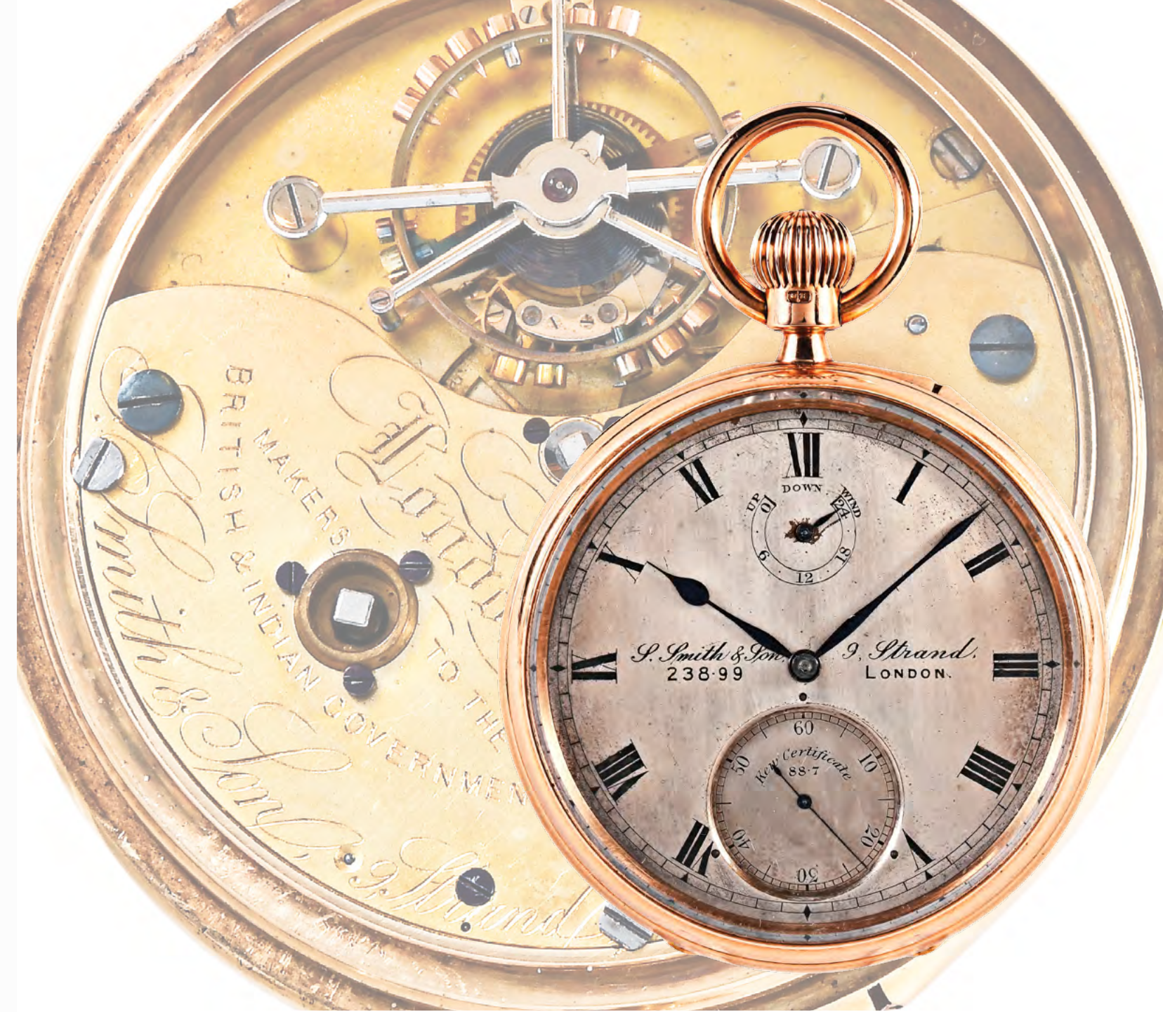
305 Nicole, Nielsen & Co. for S. Smith & Son, Clerkenwell, a late 19th century gold one minute tourbillon pocket watch, 19 jewels, stem wind and pin set, gilt half plate keyless reverse fusee movement with lever escapement, freesprung cut bimetallic balance with gold screws, three arm equidistant tourbillon carriage, and raised barrel, in an 18 karat, yellow gold, hinged back and snap bezel open face case with swivel pendant and monogram on back, London hallmark, date letter for 1899 - 1900, and "SS" sponsors mark, roman numeral silver dial with wind indicator, the seconds bit engraved "Kew Certificate 88.7", blued steel spade and poker hands, serial #238-99, 56mm, 181.4g TW, dial and movement signed
